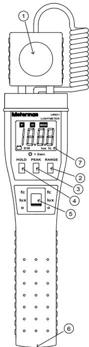
This instrument is a portable easy use 3½ digit, compact sized digital light meter designed for simple one hand operation with the reading in lux or fc units. Its controls are: 1. Sensor Head. 2. RANGE button. 3. PEAK HOLD (50 mS pulse light) button and Back light switch. 4. DATA HOLD button. 5. Lux / fc / OFF selector 6. mV output jack. 7. LCD display.
